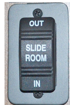
Slideout Switch (Located near the monitor panel) -Typical View
