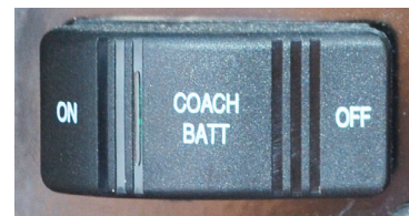
House/Coach Battery Disconnect Switch (Located near sliding entrance door)
