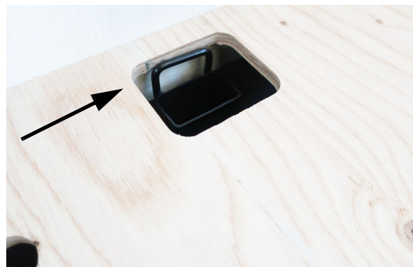
Tether Anchor Loop (Located beneath the forward facing dinette seat back cushion) dinette table must be in lowered position to use. -Typical View
